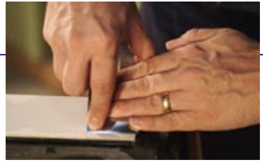
The left hand provides all the support on the bevel. The hand is spread across the width and parallel to the blade edge. The left arm is held rigid from finger tip to elbow.
