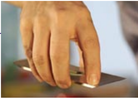
An important part of the side-sharpening process is to grip the blade correctly. The blade is grasped loosely in the right hand, held just by the fingertips.
