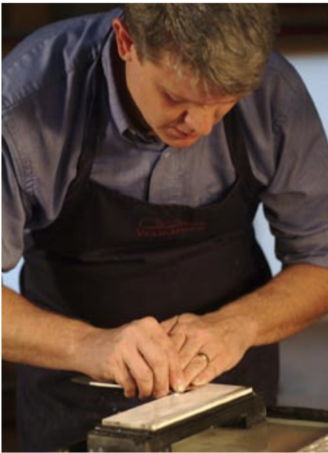
Body position is important as well. I'm standing with my head positioned directly over the blade. This puts my line of sight directly in line with the blade tip and where I'm sharpening.
